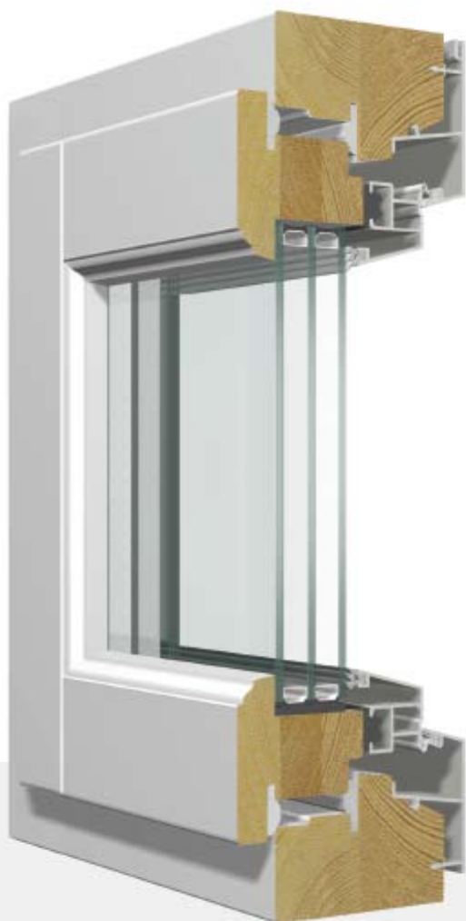
Timber-aluminium window Frame depth 105 mm U-Value down to 0,9 W/m 2 K with 2k + 1 double-glazed sash and 3k triple-glazed sash
