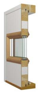
The double seals, the polystyrene insulation and the energy efficient glazing guarantee that the strongly built Skaala Tradia exterior doors have an effective thermal insulation. The reinforced structure comes with a ten year guarantee for resisting warping. The doors are delivered complete with a durable threshold of hardwood.
